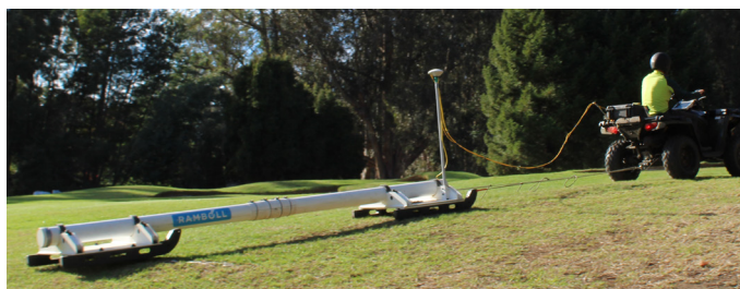
Ramboll using the electro-magnetic survey tool at the Seascape Golf Course.
