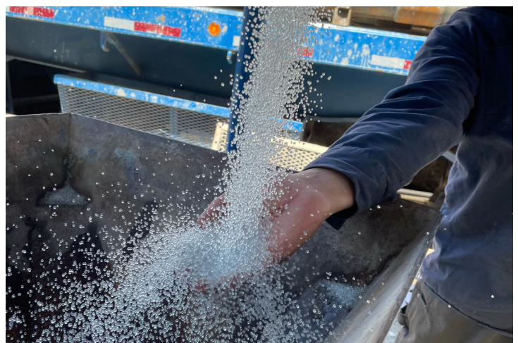
These glass beads are the packing material that goes around the well casing. They allow water to flow out into the aquifer.
